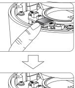
Take the micro SD card out carefully from the camera. It may cause a malfunction of the micro SD card or the micro SD card slot if you use the power too much at lock status.
