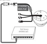
NOTE: If the camera doesn't work properly after connecting PoE device, please check if the PoE device supplies enough power.
