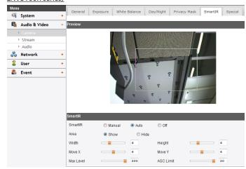
> SmartIR: SmartIR function improve the sensitivity in the low luminance. SmartIR analyze the image of the screen, when the subject is close. Then SmartIR reduce the IR LED
