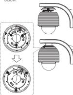
You can install the PIPE Installation Bracket direct to the other type LG Wall Mount assembly. This LG Wall Mount assembly make to easy to install your camera.
