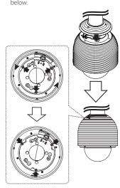
You can install the PIPE Installation Bracket direct to the other type LG Wall Mount assembly. This LG Wall Mount assembly make
