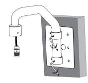
4 Install the PIPE Installation Bracket to the Parapet Mount Bracket.
