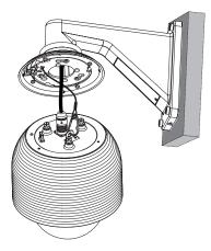
Attach the camera to the PIPE Installation Bracket by following step 1 and 2. Align the locking point of the PIPE Installation Bracket and the camera body.
