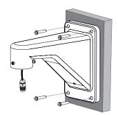
2 Install the Wall Mount Bracket to the wall.
