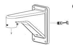
Pass the connection cable throught the Wall Mount Bracket.
