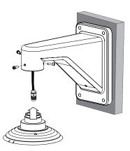
Install the PIPE Installation Bracket to the Wall Mount Bracket.
