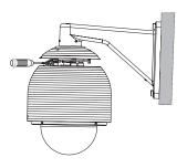
Assemble the PIPE Installation Bracket as shown below.
