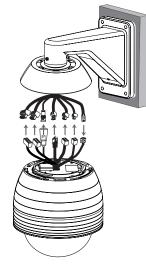
**5** Assemble the camera to the PIPE Installation Bracket by turning it clockwise. Tighten the M3 SAMS Screws and then align the cover adaptor and main body.
