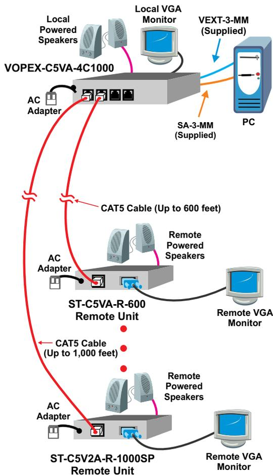
The VOPEX® VGA Video Splitter/Extender simultaneously broadcasts high-resolution VGA video from one computer to 4 or 8 remote monitors located up to 1,000 feet away using CAT5/5e/6 cable. Audio can be broadcasted to self-powered stereo speakers at the local unit and each remote location when using NTI's remote units with audio option.
