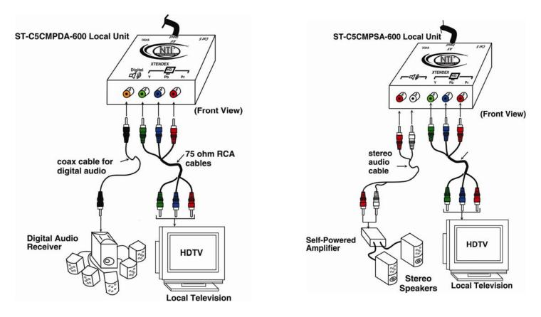
Figure 2- Connect the local television and audio device to the Local Unit
