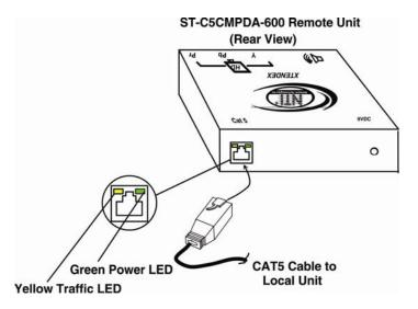
Figure 5- Connect the CAT5 cable to the Remote Unit
