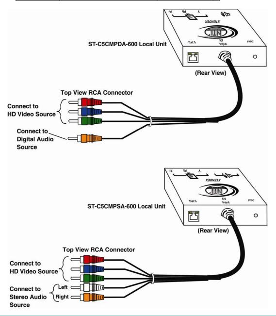
2. Connect 75 ohm RCA cables between the local HDTV and the RCA connectors marked "Y", "Pb", and "Pr" on the local unit as shown in Fig. 2.
