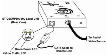
Figure 3- Connect CAT5 cable to Local Unit
