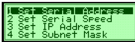
Figure 12- Configuration menu on LCD
