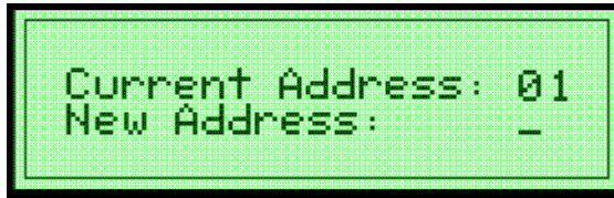
Figure 13- Set Serial Address from LCD and keypad
