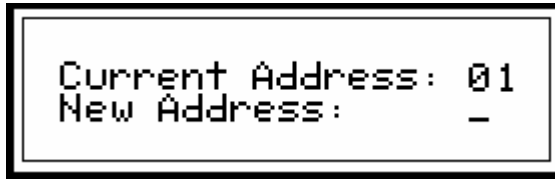
Figure 14- Set Serial Address from LCD and keypad
