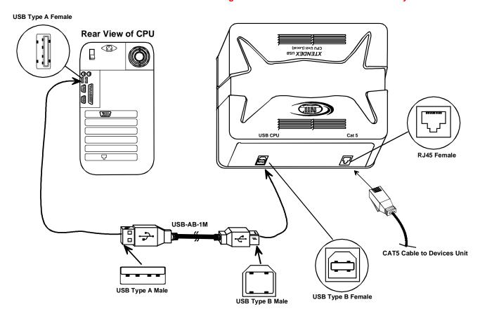
Figure 1- Connect the CAT5 USB Extender to a CPU
