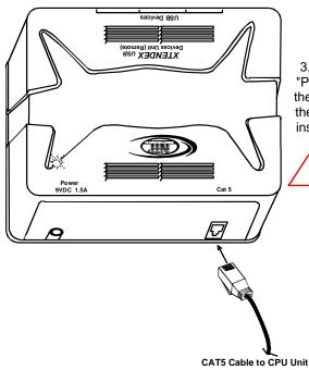
3. Make sure the CAT5 cable has been installed in accordance with the "Preparation for Installation" instructions on page 2. Connect the CAT5 cable to the "CAT5" port on the Devices Unit. (If an RJ45 wall outlet is being used, connect the other end of the extension cable to the RJ45 wall outlet.) When properly inserted the CAT5 cable end should snap into place. (See Fig. 3.)
