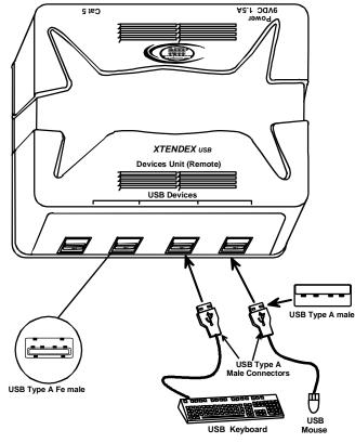
Figure 2- Connect devices to the CAT5 USB Extender
